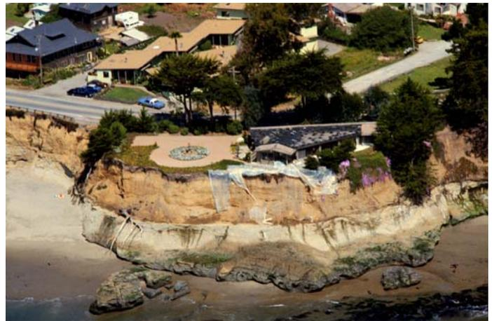
Photo 6-4. Example of bluff erosion. (Source: G. Griggs)
