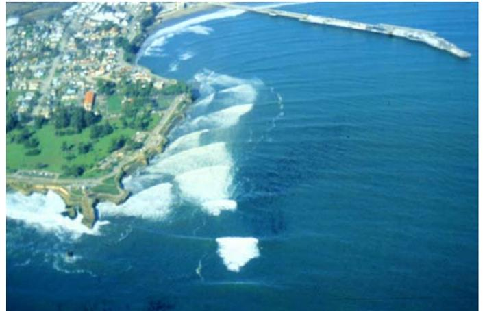
Photo 6-3. Wave refraction near Lighthouse Point. (Source: G. Griggs)
