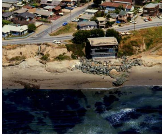
**Photo 6-9. Purisima outcrop in front of O'Neill house that serves as a natural groin, which traps littoral drift. (Source: G. Griggs)**
